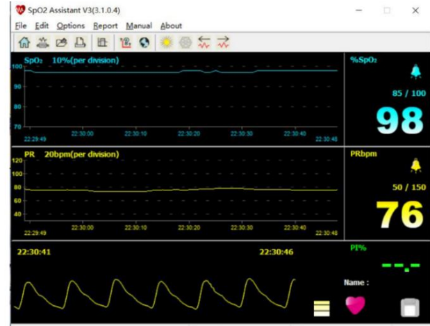
Fig. 2. Real-time monitoring dashboard showing SpO2 levels (top graph), pulse rate (middle graph), and the photoplethysmogram (PPG) waveform (bottom graph).
