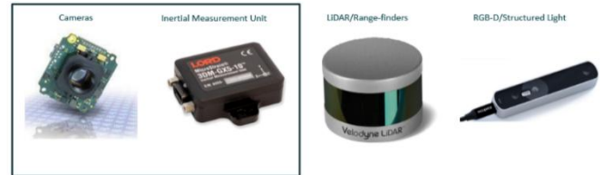
Fig. 4. Multi-sensor configuration for mobile robot navigation including camera, IMU, and 3D LiDAR modules.
