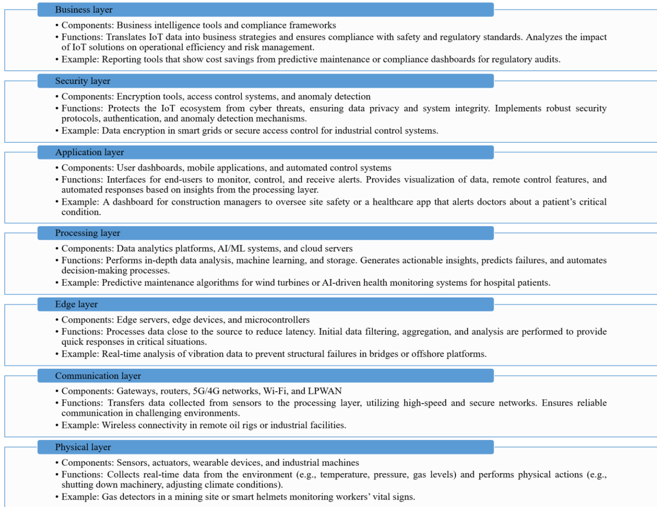
Fig. 2. Layered IoT architecture explicitly designed for high-risk environments.
