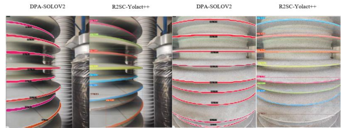
Fig. 9. Comparison of shed segmentation results of R2SC-Yolact++ and DPA-SOLOV2.
