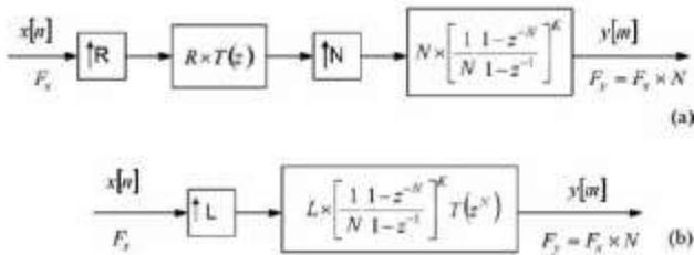
Figure 7: Two-stage interpolator composed of an FIR filter in the first stage, and the CIC filter in the second stage:
