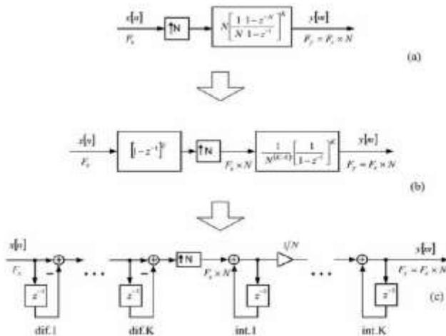
Figure 5: Block diagram representation of CIC interpolator:
