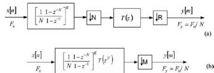
Figure 6: Two-stage decimator composed of a CIC filter and an FIR filter:
