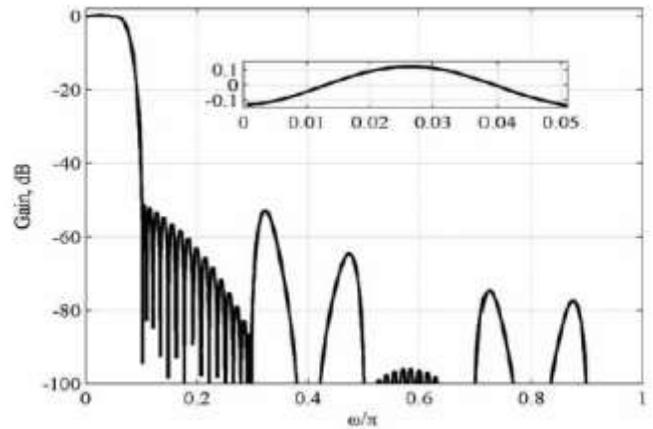
Figure 9: Gain responses of the two-stage decimator implemented as a factor of 5 and a factor of 2.
