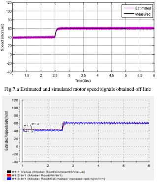
Fig 7.b Estimated and simulated motor speed signals obtained in real time
