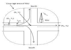
Figure 3(a). Case 1 when vehicle can take turn.
