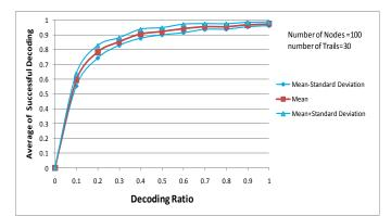
Figure.5.A WSN is randomly distributed in a field. The average of successful decoding ratio is shown for network size=100 nodes and buffer size= 10 slots with the MDSA algorithm
