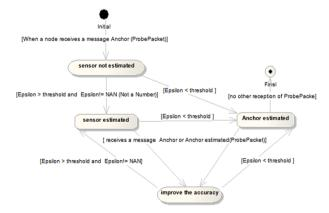
Figure 1: State machine diagram for Sensor node not estimated
