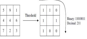
Fig.2: The basic LBP operator
