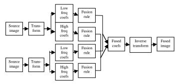
Figure 2: Block diagram of generic model of multi scale image fusion
