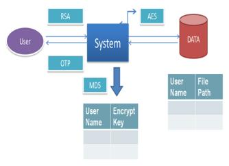
Figure 2. Proposed Security Model/ Structure
