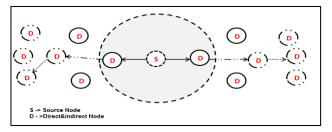
Figure 1 A WSN is randomly distributed in a field. A node **S** is source node and flood its data to its neighboring nodes D then D unicast its data to one of its neighbors and so on.
