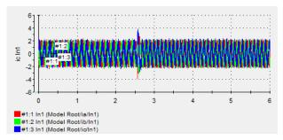
Fig. 9.a (Experimental) Motor three phase current step up of reference speed
