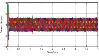
Fig. 6.b (Simulation) Motor three phase current for step down of reference speed
