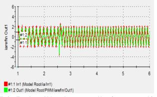
Fig 8.a (Experimental)Motor phase current and its reference command for step up of reference speed
