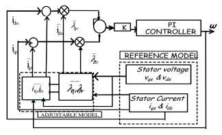
Fig. 2 Block Diagram for Speed Estimation Procedure
