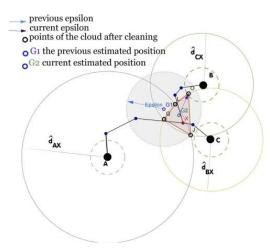
Figure 2: Example of estimating the position for X at the reception of localization information from C anchor
