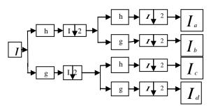
Fig 1: Structure of 2-D DWT
