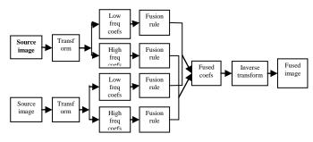
Fig 5: Block diagram of generic model of multi scale image fusion
