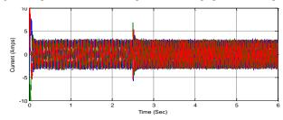
Fig. 9.b (Simulation) Motor three phase current for step up of reference speed
