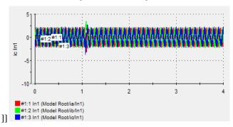
Fig. 6.a (Experimental) Motor phase current and its reference command for step down of reference speed
