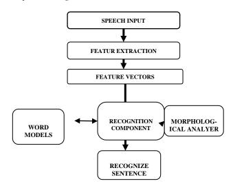
Fig. 5. Functional block diagram of the Speech Recognition Module
