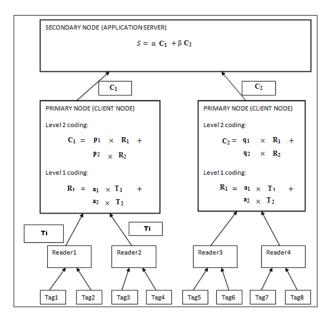
Figure 4. Architecture for Multilevel network coding
