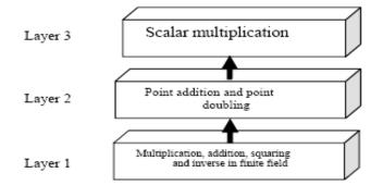
Figure 2. 3-tier architecture of ECC scalar multiplication
