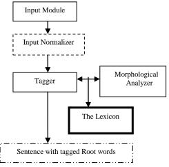
Fig. 6. Functional block diagram of the Morphological Analyzer
