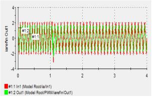
Fig. 6b (Experimental) Motor phase current and its reference command for step down of reference speed
