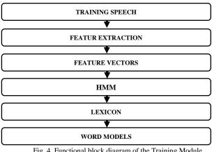
Fig. 4. Functional block diagram of the Training Module
