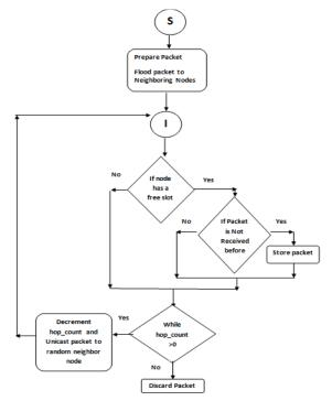
Figure.2 Modified Distributed Storage Algorithm Flowchart (MDSA)
