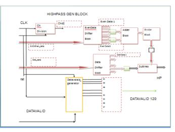
Fig 7.3 Block diagram of High pass generation block (ROW processor)
