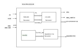
Fig 7.2 Block diagram of ROW processor
