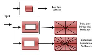
Fig 3: Block diagram of NSCT
