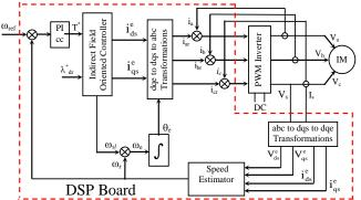
Fig. 1 Block Diagram of the Proposed Speed Sensorless Control System
