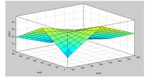
Figure 4. Surface of Compressive Strength for Cement and Flyash Content
